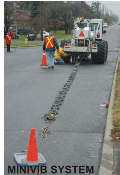
Figure 2: Photos of the SH-wave landstreamer in operation in Orleans with a) hammer/roller source, and b) minivib source.
